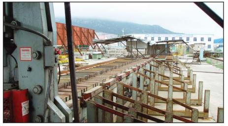
KRB Standard Shearline with pockets for straight stock and conveyors to bending stations down stream.
