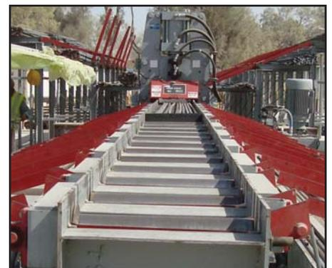
KRB Standard Shearline conveyors to bending stations down stream.
